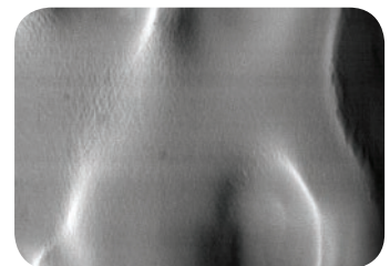
Competitor PFA Bottle Inside Base (1000x SEM Magnification)
